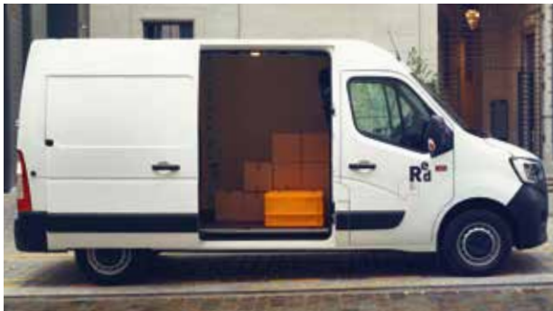
SIDE DOOR WIDTH UP TO 1,270 MM for loading europallets.
