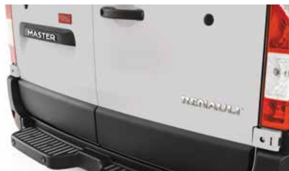
REAR ACCESS STEP from 542 mm.
