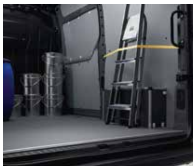
6 mm polypropylene side walls and non-slip floor
