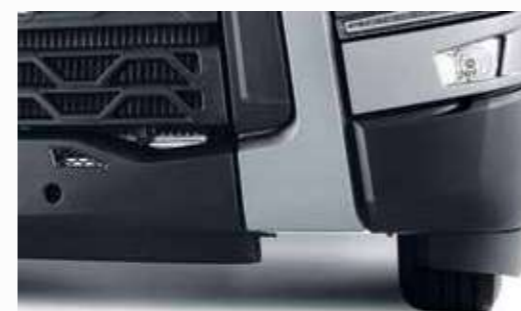
AERODYNAMIC BUMPER EXTENSIONS to improve air penetration.
