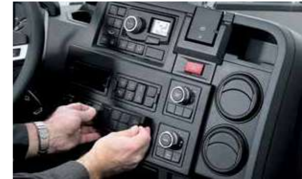
SWITCH LOCATIONS CAN BE CHANGED to customise the driving position.
