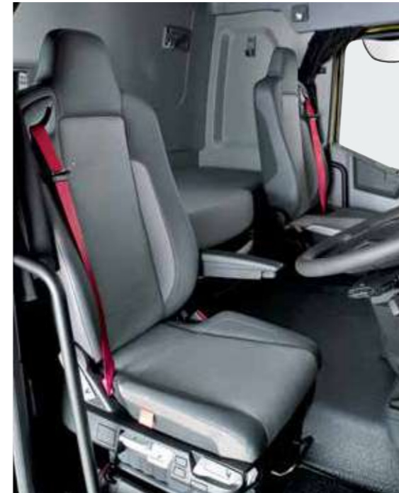
AIR-SUSPENDED SEATS with integral seat belts, head rests. Ventilated and heated seats* side and lumbar support adjustment; slide adjustment range of 20 cm*.
