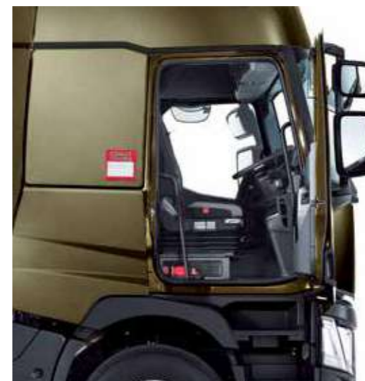
DOOR OPENING ANGLE 85° for easier cab access.
