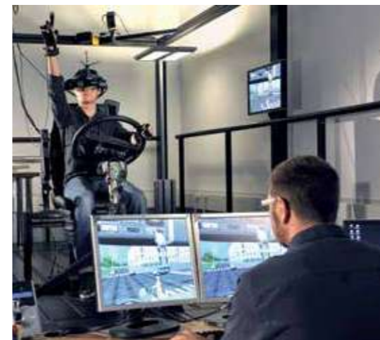
VIRTUAL REALITY to optimise the ergonomic layout of the driving position.
