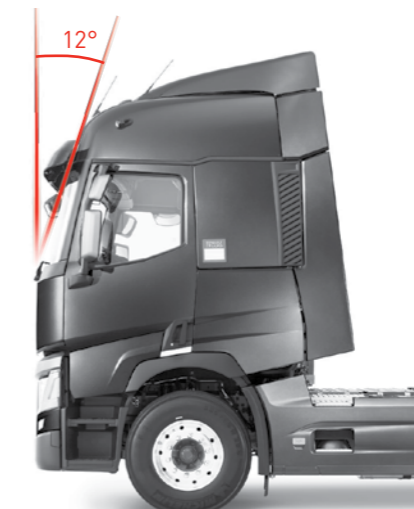
12° INCLINED WINDSCREEN for a better aerodynamic profile.
