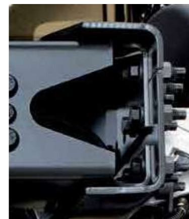
SIDE MEMBER REINFORCEMENTS to suit application.
