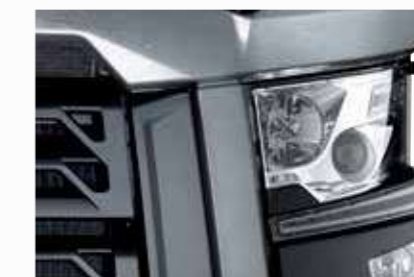
DEFLECTOR INTEGRATED IN HEADLAMP UNIT to deflect the flow of air.
