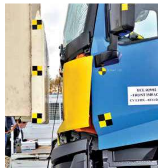
FRONTAL IMPACT to measure the impact resistance of the cab.
