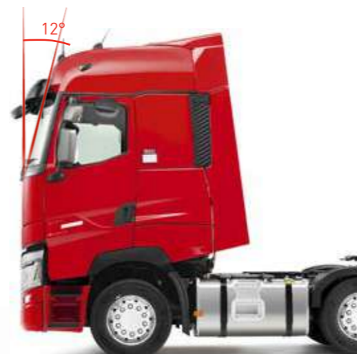
12° INCLINED WINDSCREEN for a better aerodynamic profile.
