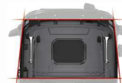
TRAPEZOID-SHAPED CAB 2.3 metres at the front and 2.5 metres at the rear to improve air flow.
