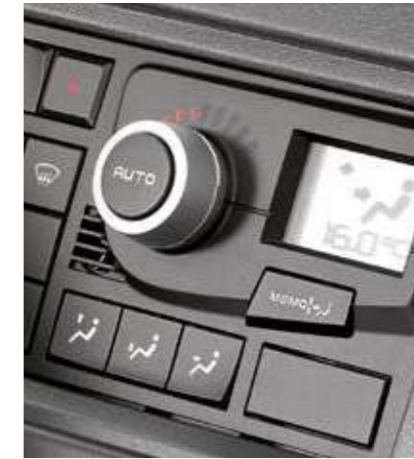
AIR CONDITIONING AND AUTOMATIC DE-FROSTING of the side windows, windscreen and rearview mirrors.
