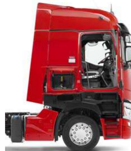
DOOR OPENING ANGLE 85° for easier cab access.
