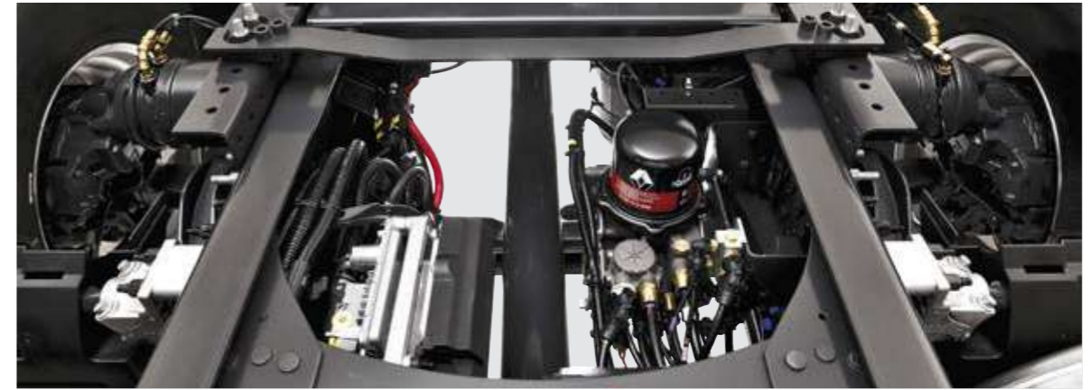
SEPARATION OF WIRING HARNESSES AND AIR PIPES for easier maintenance.
