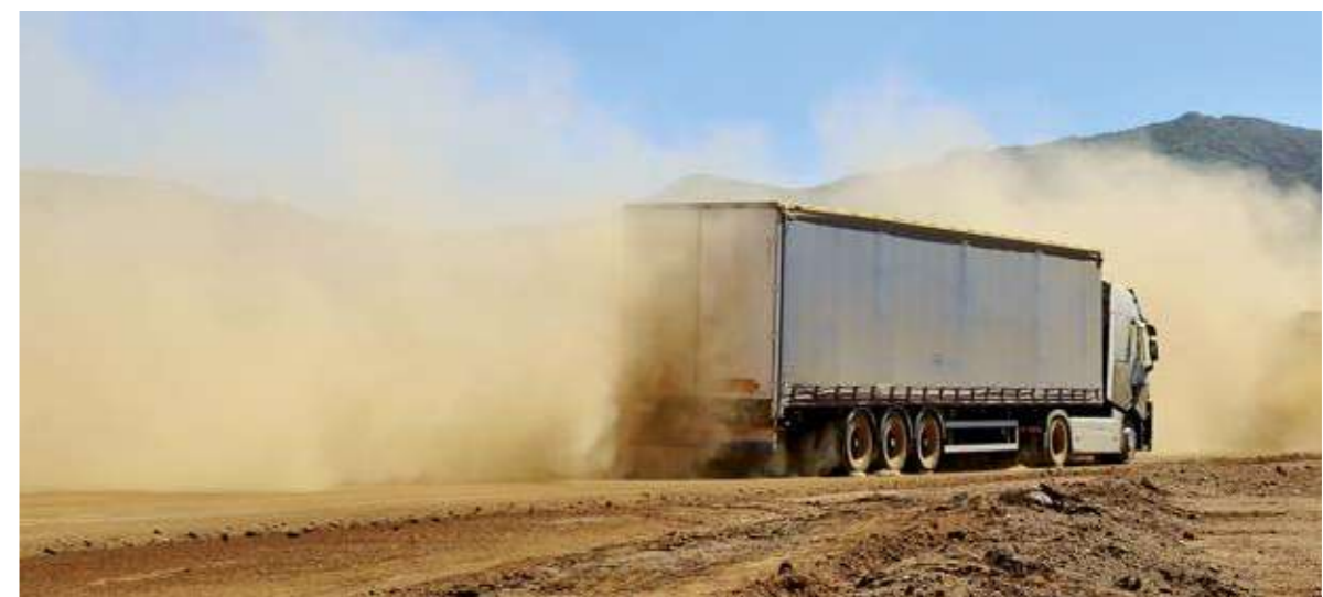
EXTREME TEMPERATURE TEST in Almeria, Spain to measure vehicle resistance to harsh conditions (dust, heat, etc.).
