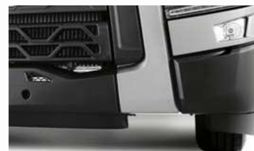
AERODYNAMIC BUMPER EXTENSIONS to improve air penetration.
