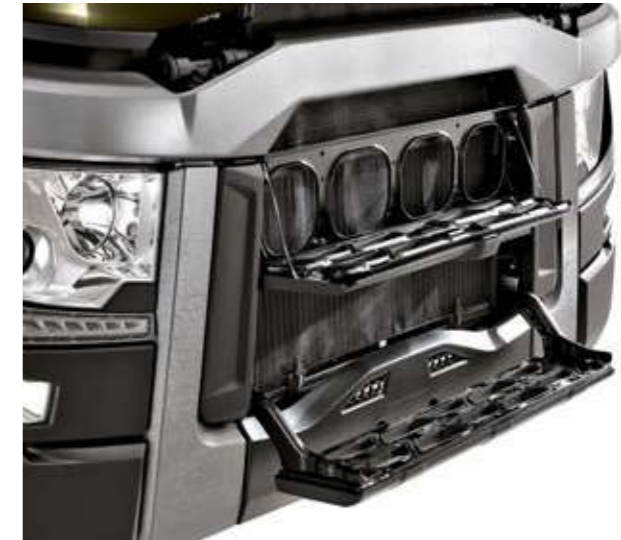
WINDSCREEN ACCESS STEPS via two platforms for cleaning the windscreen.
