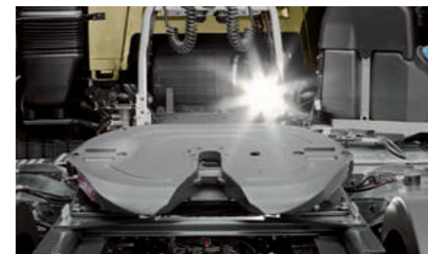
WORK LIGHT to light up the platform.
