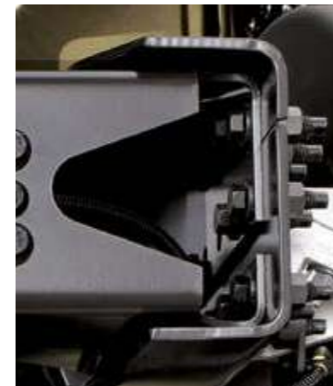
SIDE MEMBER REINFORCEMENTS to suit application.
