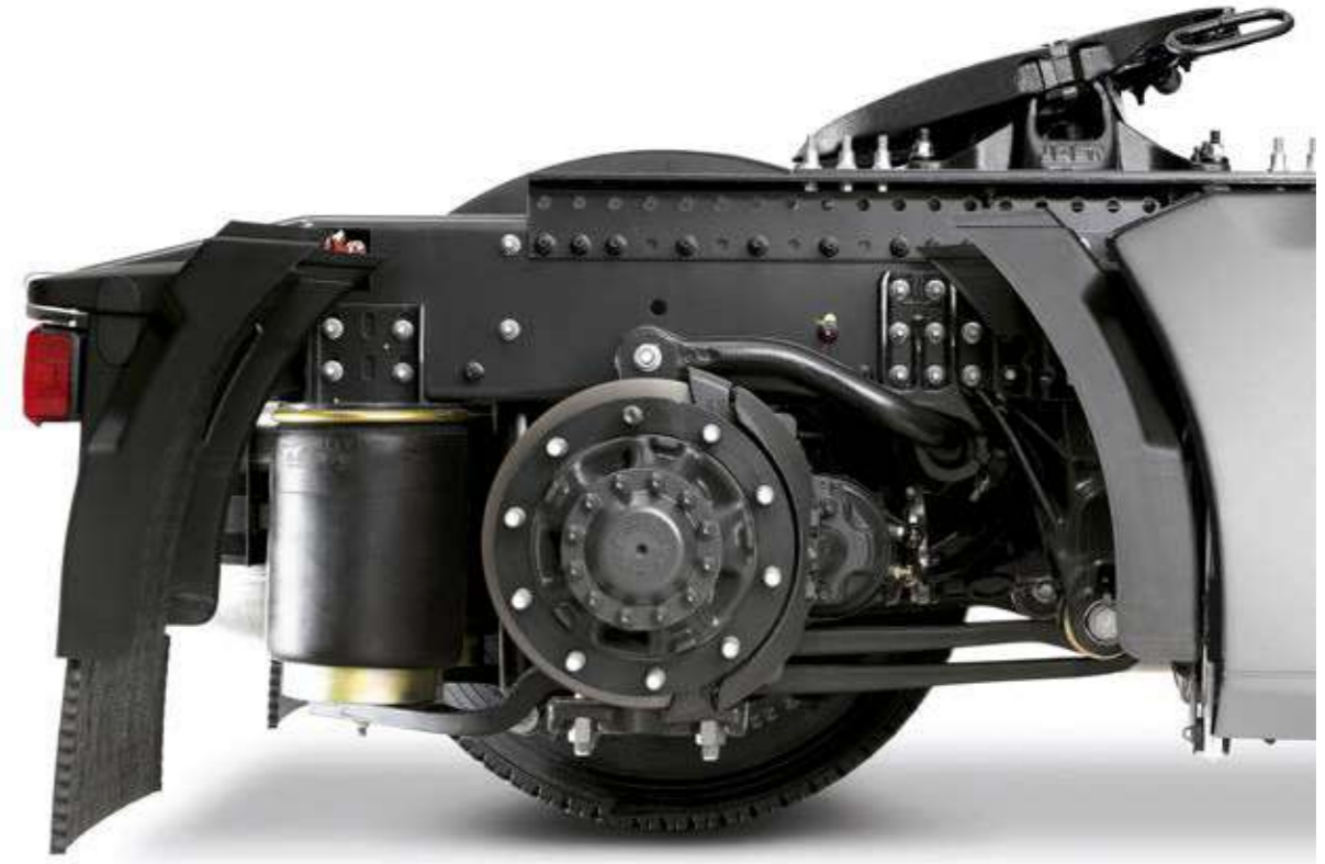
REAR AIR SUSPENSION design capacity 13 t.
