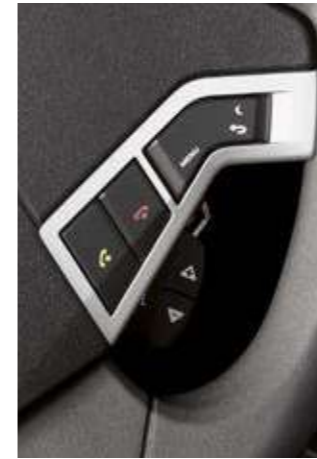
STEERING WHEEL-MOUNTED CONTROLS for telephone and menu navigation.
