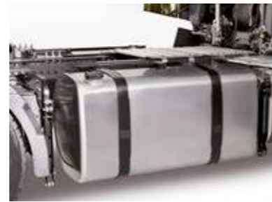
CAPACITY UP TO 1,475 L for extended operating range.
