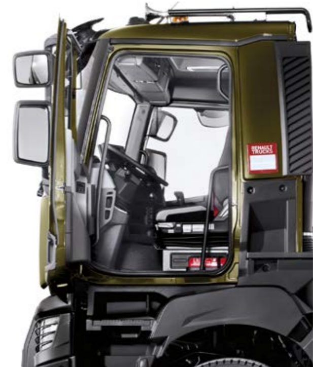
DOOR OPENING ANGLE 85° for easier cab access.
