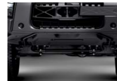
GUARD PLATE underneath the radiator and oil sump.
