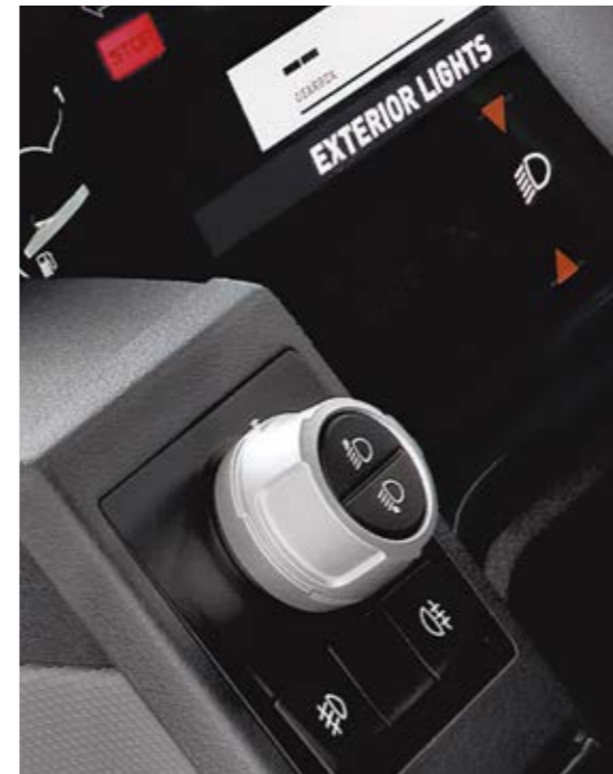
ROTARY BUTTONS within reach and easily readable information on the information display.
