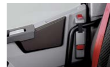
MECHANICAL DOOR LOCKING for additional door closing from inside the vehicle.
