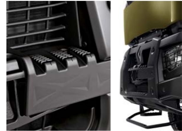
WINDSCREEN ACCESS STEPS non-slip to make servicing the vehicle easier.
