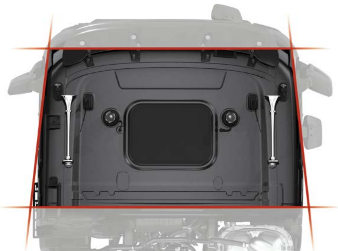
TRAPEZOID-SHAPED CAB for better air penetration and better handling.
