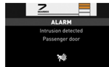
INTRUDER ALARM warns the driver if the doors are opened.
