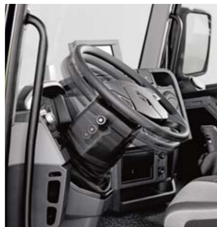
STEERING WHEEL ADJUSTABLE IN THREE DIMENSIONS height, depth and rake.
