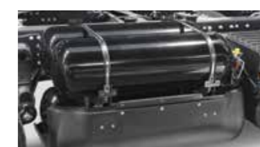
NATURAL GAS (CNG) STEEL TANK with a gas capacity of up to 120 kg.
