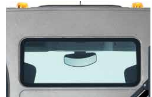
CAB REAR WINDOW to assist with handling equipment (tipper, platform, etc.).
