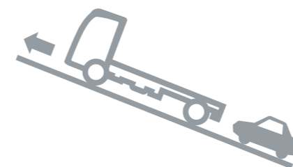
HILL START AID brakes are held on to prevent the truck rolling backwards.
