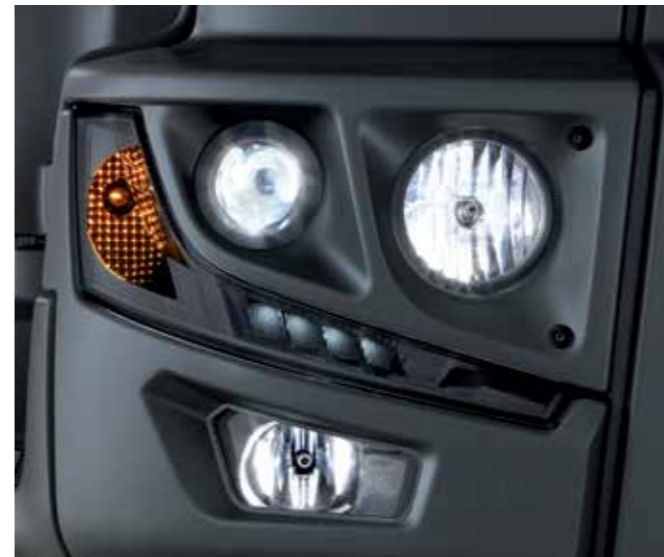
LIGHTS equipped with daytime running lights with 4 LEDs.
