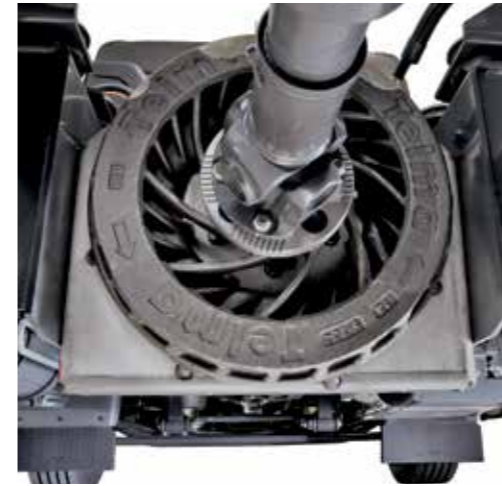
ELECTRIC RETARDER IN DRIVELINE and hydraulic retarder on gearbox.
