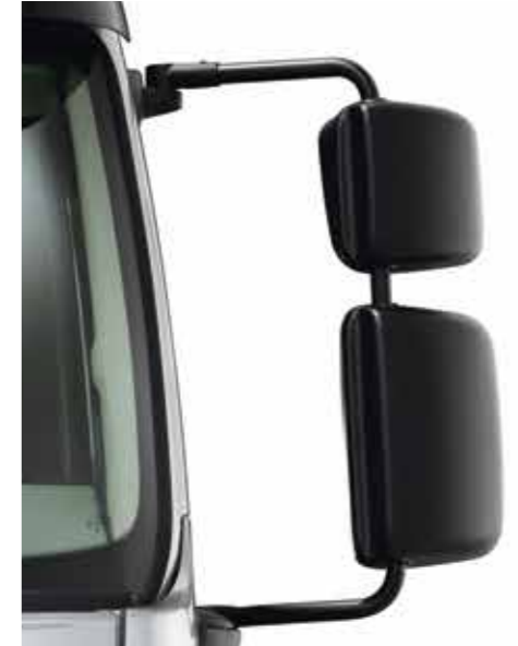
REARVIEW MIRRORS suitable for different cab widths with reinforced brackets to reduce vibration.
