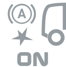
AUTOMATIC EMERGENCY BRAKING SYSTEM possible collision warning followed by braking to bring the vehicle to a complete standstill without the driver's intervention.
