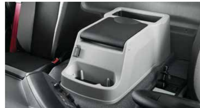
CENTRAL STORAGE COMPARTMENT capacity 15 L, writing surface, bottle holder, cupholder and supplementary 24 V power supply.
