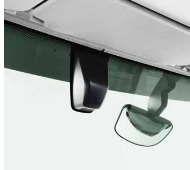
CAMERA for the line crossing warning and automatic emergency braking.
