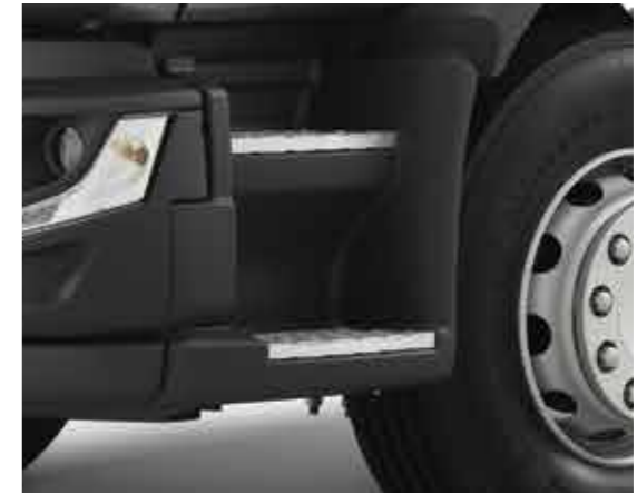
STAIRCASE TYPE STEPWELL with an 80 mm recess between the two steps for easier cab access.
