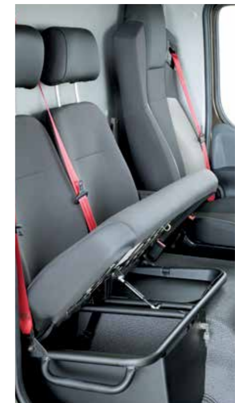
STORAGE UNDER BENCH SEAT with liftable seat cushion.
