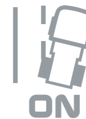
LANE DEPARTURE WARNING SYSTEM warns the driver with an audible alarm if an unintended deviation of the vehicle's direction is detected.
