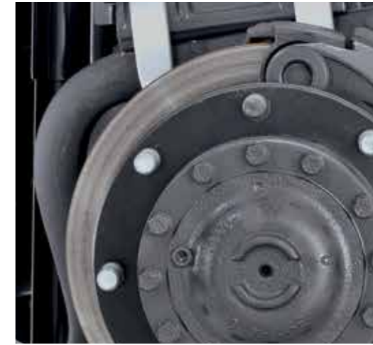
DISC BRAKES provide emergency braking deceleration to 7 m/s 2 (the requirement is 4.5 m/s 2 ).
