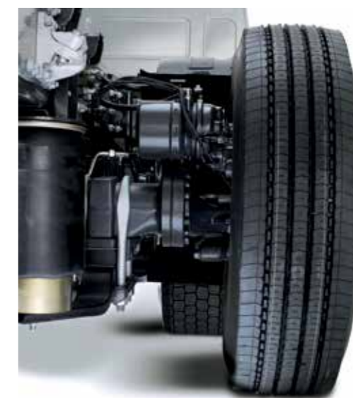
REAR AIR SUSPENSIONS offer increased stability and improved protection of goods.
