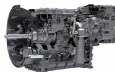
OPTIDRIVER AND OPTITRONIC GEARBOXES 7% fuel saving compared to a manual gearbox.
