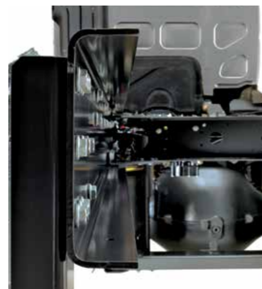
CHASSIS SIDE MEMBERS in high tensile steel.
