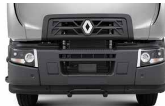
BUMPER WITH STEEL CORNERS (D WIDE) for greater resilience.
