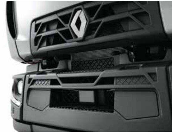
WINDSCREEN ACCESS STEPS non-slip to make vehicle servicing easier.
