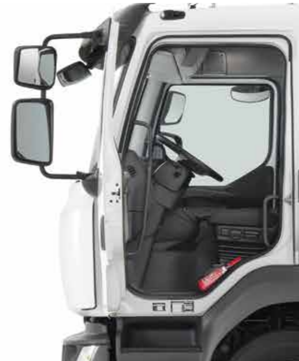
90° OPENING for easier cab access.
